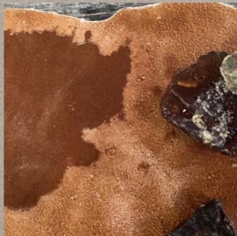
Sanding and polishing using goat skin
